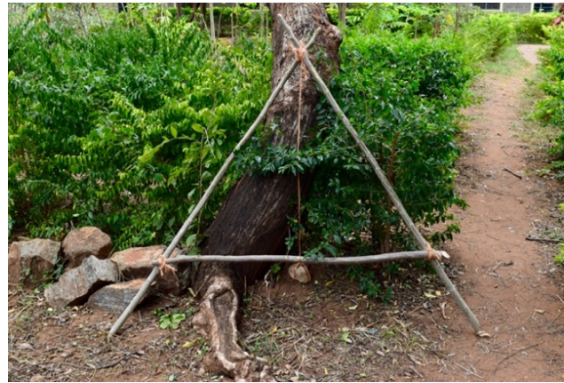
Figures 5a & 5b. Top left, Mr. Joseph Mwanganda. Bottom right. A level made from sticks, a rock and sisal rope.
